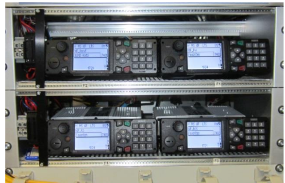
Abb. 113 Fixed Radio Terminal (FRT)
